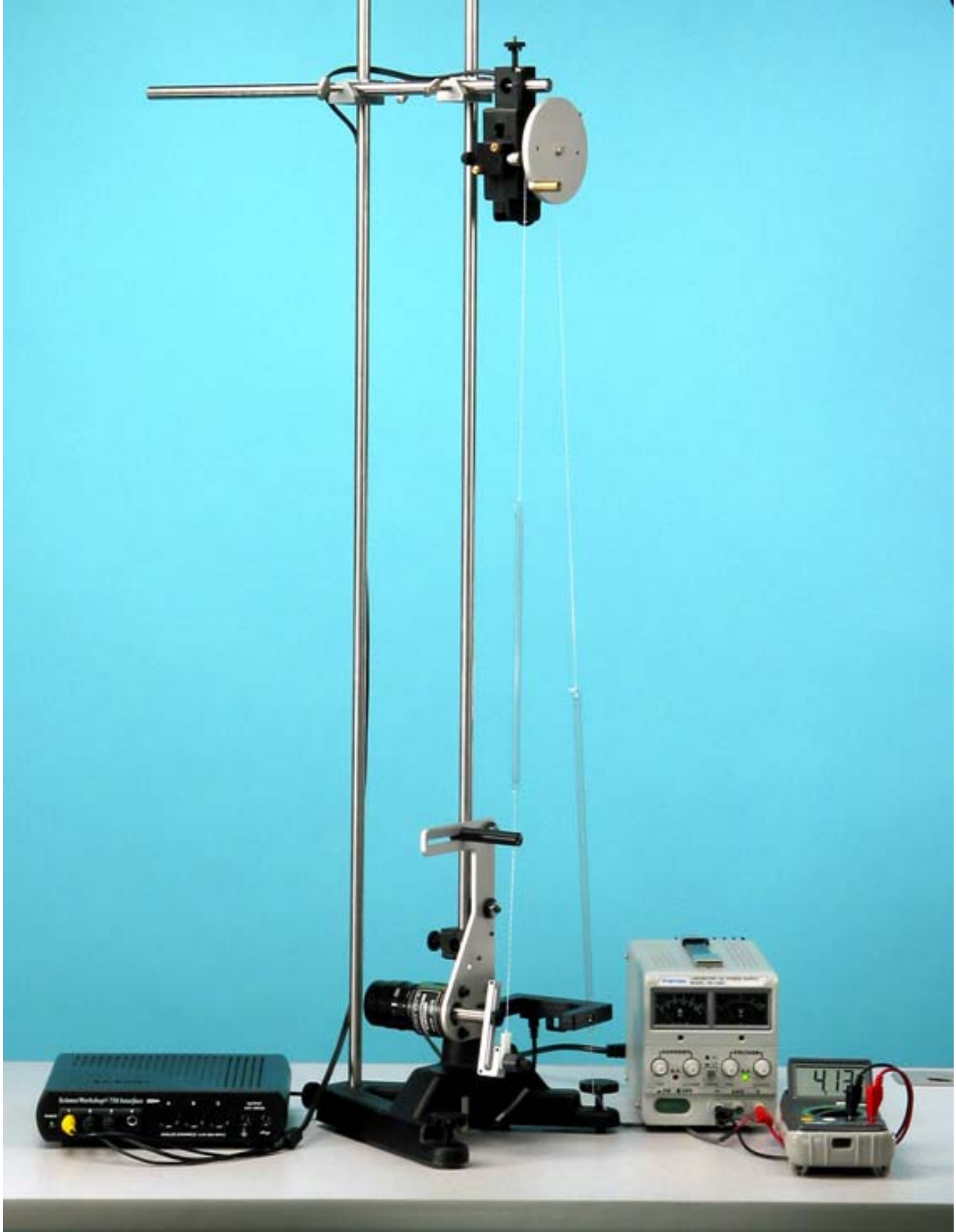
Figure 6: Experimental driven pendulum. This angular motion of the round metal pendulum at the top is expected to exhibit chaotic motion. [2]
