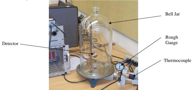
For your protection, cover the bell jar with the protective metal cover before pumping down; this will prevent glass shards from flying in the (unlikely) event the jar shatters under vacuum.
