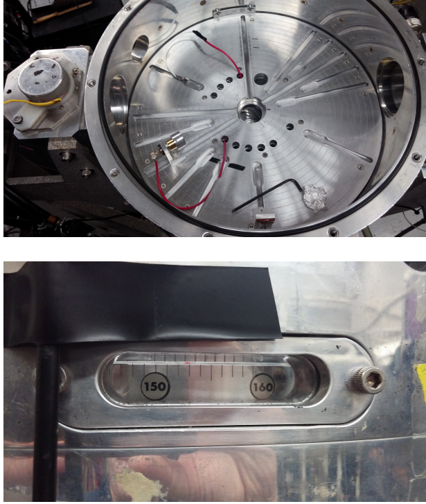
Figure 2: The detector was positioned at 149.95^\circ \pm 0.05^\circ relative to the direction of the proton beam. This angle was maintained through both experiments.
